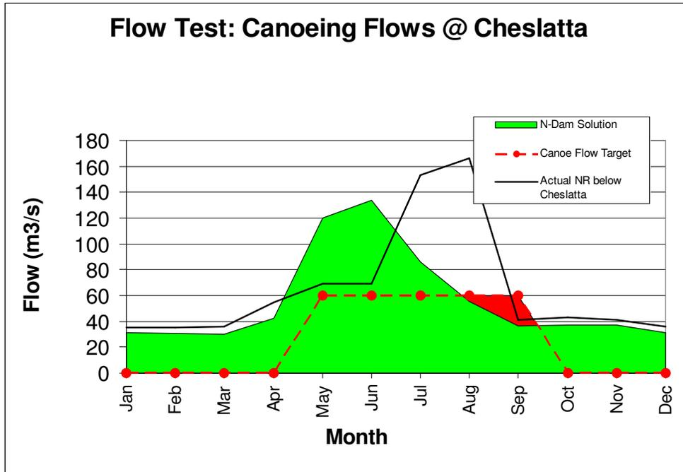
Figure 6. Example of flow test: comparison of the N-DAM solution (blue line) with Cheslatta sturgeon flows (black line). The pink area shows the difference between the two flow regimes.
