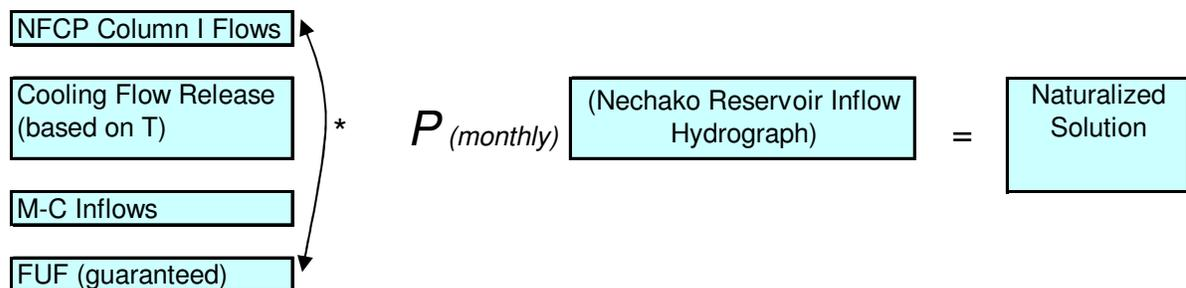
The target temperature implies a choice of Water Release Facility (WRF) that in turn determines both the amount of cooling flow required, and the resultant Freed-Up Flow (FUF) that will be remaining. The model allows the option for some of the FUF to remain in the reservoir. After choosing the desired temperature target, WRF design, and flow inputs, the model redistributes the flow into the Nechako River system, generates hydrograph figures, and assesses the fit to stakeholder interests.
