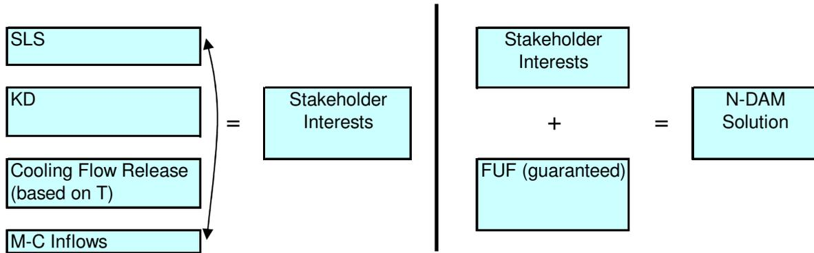
The naturalized flow redistribution is calculated as the sum of NFCP Column 1 flows, the cooling flow release, and the M-C inflow, plus the FUF guaranteed flows, weighted by the Nechako Reservoir Inflow Hydrograph. The weighting results in the same mean annual flow as for the N-DAM release, however, mean monthly flows are altered so that their pattern matches the natural flow regime.
