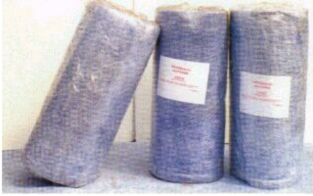
Plate 1. Mat-Sorb pads used to test storm sewer waters for the presence of petroleum hydrocarbons.
